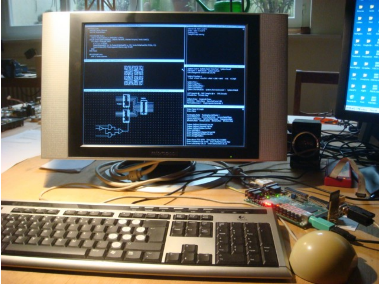
Figure 3.1 Typical Oberon display configuration with tool track on the right
